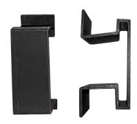
The RJC-SG Clip series (patent pending) is specifically designed for Strongwell's Strongirt composite z-girts. The .040" thick polymer clips offset insulation from the face of the girt creating airflow for rear ventilating rain screen systems.
