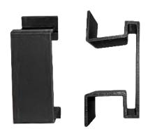
The patented RJC-SG Clip series is specifically designed for Strongwell's Strongirt composite z-girts. The .040" thick polymer clips offset insulation from the face of the girt creating airflow for rear ventilating rain screen systems.
